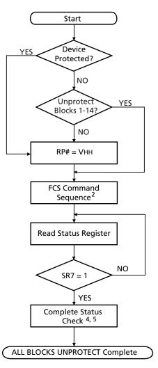
**NOTE:** 1. Once the device protect bit is set, it can be reset.
