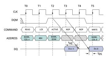
**NOTE:** A CAS latency of three is used for illustration. The READ command may be to any bank, and the WRITE command may be to any bank.
