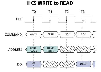
NOTE: A CAS latency of two is used for illustration. The WRITE command may be to any bank and the READ command may be to any bank. DQM is LOW. For more details, refer to Truth Tables 4 and 5.
