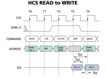
NOTE: A CAS latency of three is used for illustration. The READ command may be to any bank, and the WRITE command may be to any bank. If a CAS latency of one is used, then DQM is not required.
